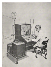
BioActivity Monitor Continuous observation of biological reactions; direct non-destructive recording of metabolic events
